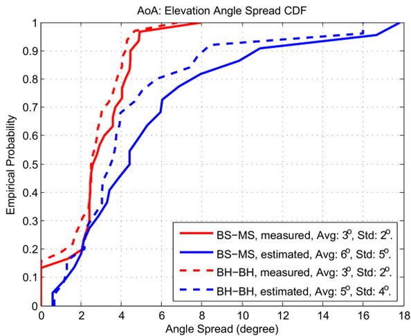
Fig. 6. Measured vs estimated AoA elevation angle spread.
