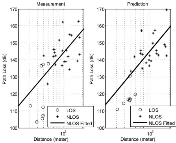
Fig. 3. Measured vs estimated path loss in base-station-to-mobile scenario for all measured RX locations. The comparisons in path loss exponent are made for the case of the ray tracer using identical locations and antenna patterns, and using the best pointing angles for single beam antennas at each location, just as was measured and presented in [1], [2]. Here, we combine all TX heights as multiple measurements for a given RX location, and pick the best pointing angles for a fair comparison.
