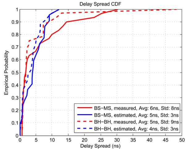
Fig. 4. Measured vs estimated delay spread of the mmWave channel. Avg indicates average value, and Std means standard deviation.
