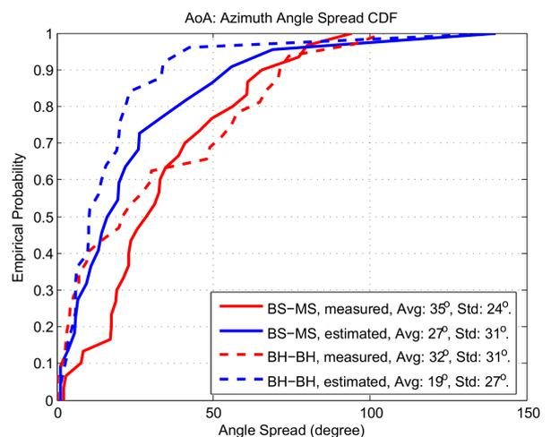
Fig. 5. Measured vs estimated AoA azimuth angle spread.
