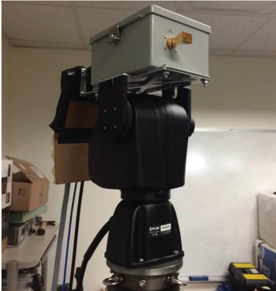
Fig. 1: 73 GHz channel sounder RF front-end up-converter with a 20 dBi gain (15° beamwidth) directional horn antenna (used for indoor measurements in a typical office environment), mounted to a degree-precision LabVIEW-controlled FLIR gimbal. The gimbal is mounted to a pneumatic mast that lifts the RF front-end to backhaul heights up to 4 m.
