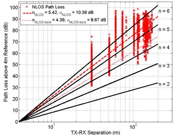
Fig. 2. Measured path loss values relative to 4 m free space path loss for 28 GHz outdoor cellular channels. These path loss values were measured using 24.5 dBi narrow beam antennas for 16 NLOS TX-RX location combinations with TX heights of 7 m and RX heights of 1.5 m. The values in the legend represent the PLEs and shadow factors, where NLOS-best represents the single best RX pointing angle at each location combination.
