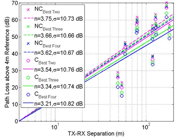
Fig. 7. Path loss versus T-R separation at 73 GHz in NYC for the best (i.e. strongest) two, three and four beams combined noncoherently and coherently at each RX location for 11 NLOS TX-RX location combinations with TX heights of 17 m and RX heights of 4.06 m. The values in the legend represent the PLEs and shadow factors for each kind of beam combination, "NC" denotes non-coherent combining, and "C" means coherent combining.
