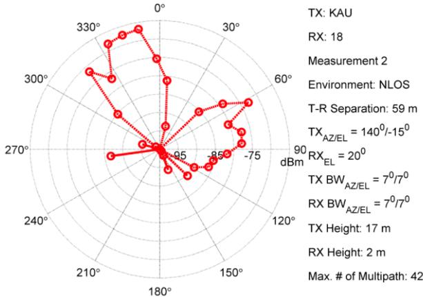
Fig. 1. Polar plot showing the received powers at a NLOS location at 73 GHz with TX heights of 17 m and RX heights of 2 m and 59 m TX-RX separation. The red dots represent total received powers in dBm at different RX azimuth pointing angles.
