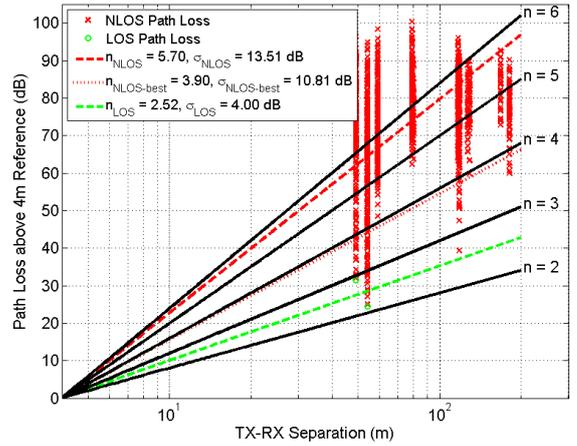
Fig. 6. Measured path loss values relative to 4 m free space path loss for 73 GHz outdoor cellular channels. These path loss values were measured using 27 dBi narrow beam antennas for 11 TX-RX location combinations with TX heights of 17 m and RX heights of 4.06 m. The values in the legend represent the PLEs and shadow factors, where NLOS-best represents the single best RX pointing angle at each location combination.
