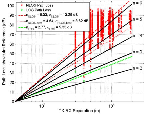
Fig. 4. Measured path loss values relative to 4 m free space path loss for 73 GHz outdoor cellular channels. These path loss values were measured using 27 dBi narrow beam antennas for 19 TX-RX location combinations with TX heights of 7 m and RX heights of 2 m. The values in the legend represent the PLEs and shadow factors, where NLOS-best represents the single best RX pointing angle at each location combination.
