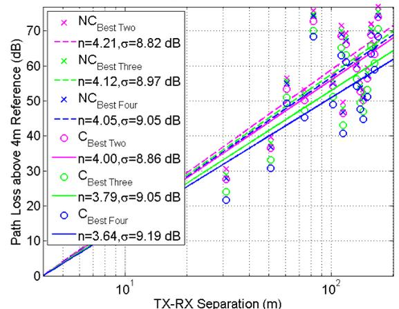
Fig. 3. Path loss versus T-R separation at 28 GHz in NYC for the best (i.e. strongest) two, three and four beams combined noncoherently and coherently at each RX location for 16 NLOS TX-RX location combinations with TX heights of 7 m and RX heights of 1.5 m. The values in the legend represent the PLEs and shadow factors for each kind of beam combination, “NC” denotes non-coherent combining, and “C” means coherent combining.
