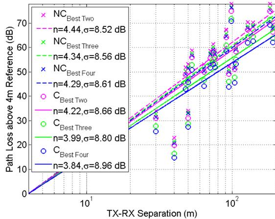
Fig. 5. Path loss versus T-R separation at 73 GHz in NYC for the best (i.e. strongest) two, three and four beams combined noncoherently and coherently at each RX location for 19 NLOS TX-RX location combinations with TX heights of 7 m and RX heights of 2 m. The values in the legend represent the PLEs and shadow factors for each kind of beam combination, "NC" denotes non-coherent combining, and "C" means coherent combining.
