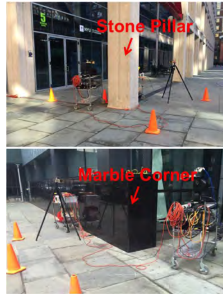
Fig. 2: TX and RX locations for outdoor diffraction measurements on the NYU campus. The test locations include a stone pillar with rounded (cylindrical) edges and a marble corner with a straight (90°) edge.
