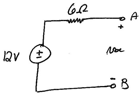
$V_{oc} = ?$  measure voltage from A to B = 12V
