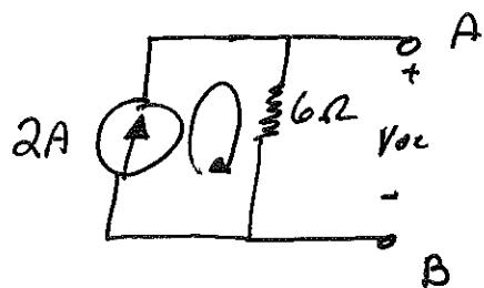
$V_{oc} = ?$  measuring  $V_{oc}$  from nodes A+B is the same as measuring the voltage across the 6Ω resistor (because in parallel)
